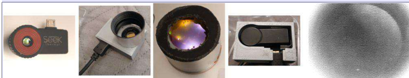
A Seek Compact Pro mobile phone thermal imaging camera adapted to fit onto a Newtonian scope using laser cutter lens eyepiece projection. (Right) A thermal IR image of the total lunar eclipse from 2007 Mar 03 taken through a 20cm Newtonian, using a different, less sensitive thermal IR camera – the bright hot spot is Tycho crater as it retains its heat inside the earth's shadow, longer than the surrounding surface.
