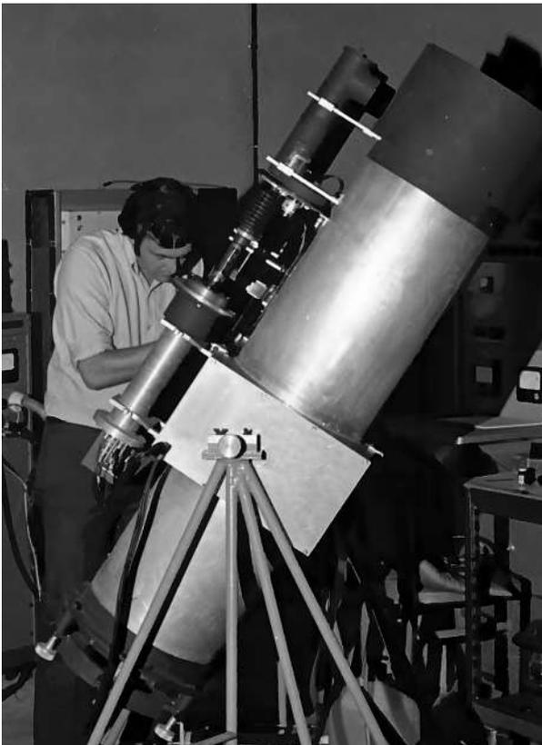
*Dr Michael Ottway working on a LIDAR (Light Detection And Ranging) instrument, c. 1972.*
